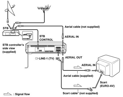
\* If your TV does not have a Scart (EURO-AV) connector, the Scart cable connected to the VCR is not required.
